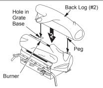
Figure 30 - Installing Back Log (#2) (Base may very from illustration)
